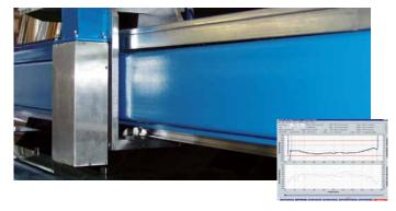
**FLOATSCAN-Coldgauge** stands for reliable and accurate inline thickness, width, and stress measurements. The gauging module's performance allows for precise thickness control, resulting in reduced profile losses when production is close to lower tolerance limits as well as minimized edge losses by accurate ribbon-width measurement. The stress module enables for optimized operation of the cooling lehr, providing additional information on the production process.
