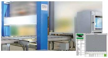
**P2-3D** based on the patented stereo-defelectometry technology - the flatness and shape of glass sheets can be measured reliably down to the m-range within less than 10 seconds. The measurement result is presented as full surface height map and additionally as avertical and horizontal curvature map.
