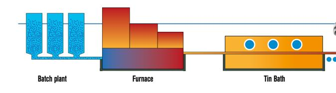
**FLOATSCAN-Hotgauge** stands for non-contacting, high-accuracy glass thickness measurement in the flow direction at the earliest possible process stage: right after the floatbath or immediately upstream of the annealing lehr. Because of its outstanding reliability, accuracy and performance, the system is a major contributor to increased production output.
