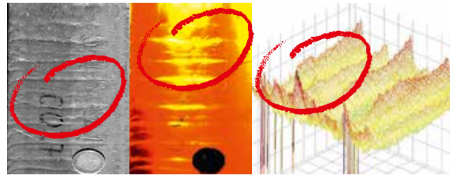
Sophisticated 2D inspection & innovative 3D technology combined – reliable defect detection on the slab surface
