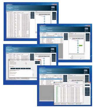
Central Recipe Tool with change log, version control, recipe comparison, and automatic recipe roll-out after release allows centralized management and tracking of all inspection systems.
